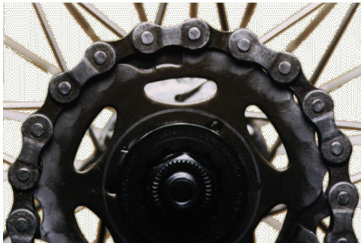
Worn chain and sprocket; still fitting together OK but starting to see daylight under some of the chain links.
