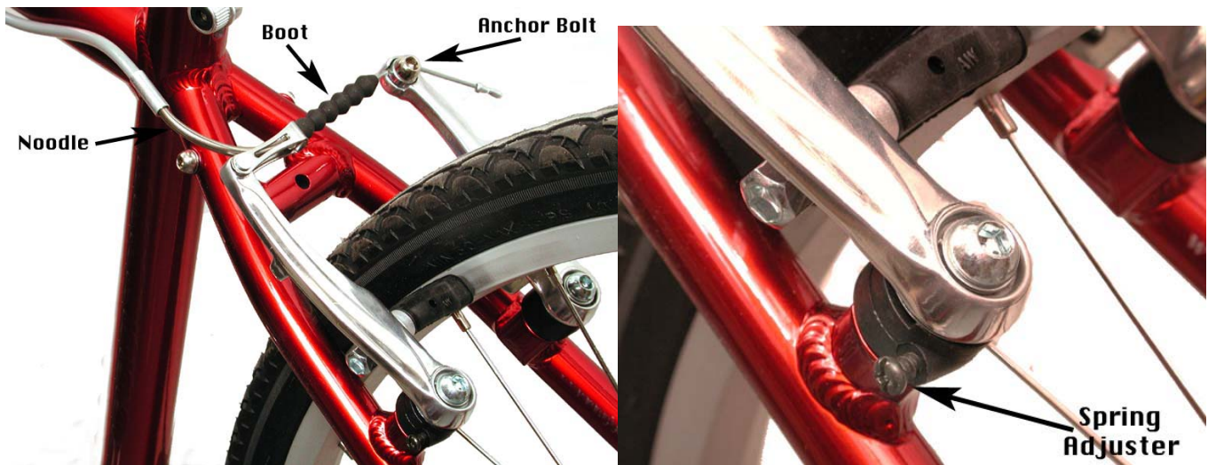
Above illustrations show a very common brake these days: direct-pull cantilever brakes AKA “V-brakes”
